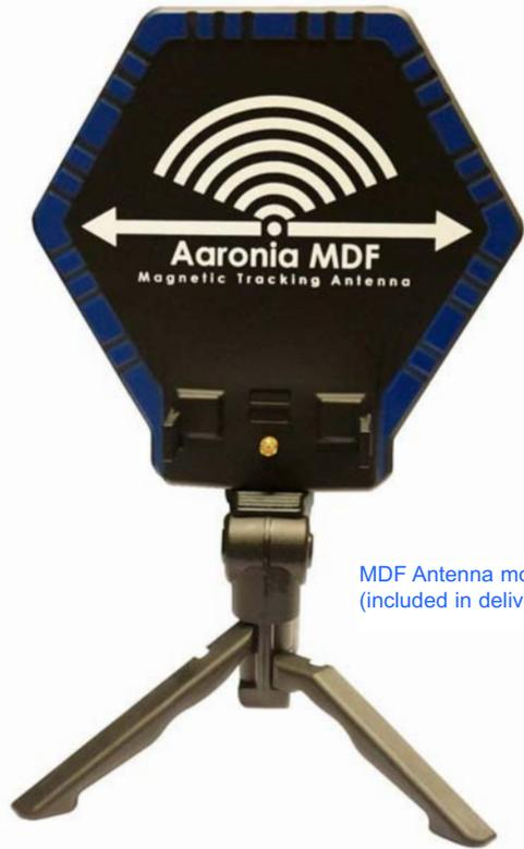
MDF Antenna mounted on mini-tripod (included in delivery)
