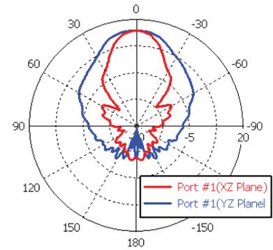
3D radiation patterns can be obtained by rotating the DUT, measuring Theta polarization and Phi polarization by angle, and summing the same location value. When the measured gain value is plotted in three dimensions, it's also possible to graph the appearance of the radiation pattern. (Antenna measurement method)
